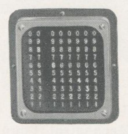
The TM-16 Digital Display Unit. If desired, the information can be fed directly to an automatic printer, typewriter, paper tape printing, adding machine printer, etc., for permanent recording.
