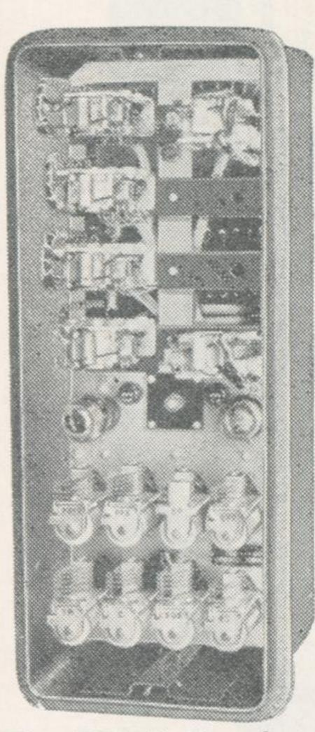
The TM-16 Receiver showing the plug-in mounted relays.
