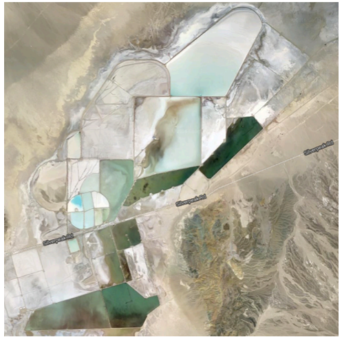
Lithium evaporation ponds at the Rockwood Lithium Mine
